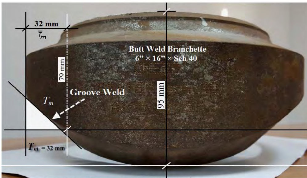
Butt Weld Branchette - 6" × 16" × Sch 40
