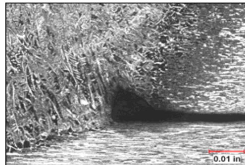
Photo 9: Mag: 50X; Etchant: Hot HCl solution Weld underfill condition
