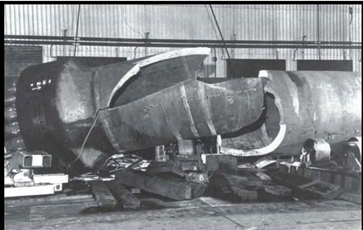
Figure 1. Brittle fracture of a steel pressure vessel during proof test. (The vessel walls were 149 mm thick, and a 2-tonne fragment was thrown 46 m). Courtesy TWI.
