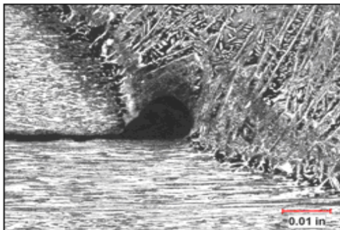
Photo 9: Mag: 50X; Etchant: Hot HCl solution Weld underfill condition
