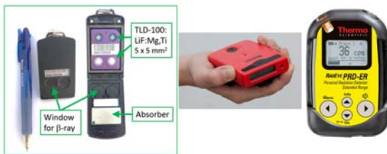
Photos of several personal dosimeters: Left: pocket passive TLD dosimeter; middle: Geiger-Müller tube based active dosimeter; right: NaI(Tl) scintillator based active dosimeter.
