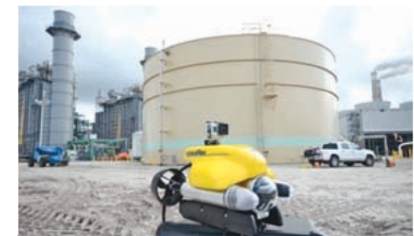
شکل ۶- Submersibles Water Tank Inspection
